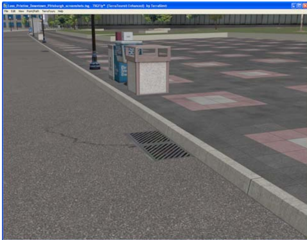
Fig. 9: Integrated sewer grate aligned to curb
