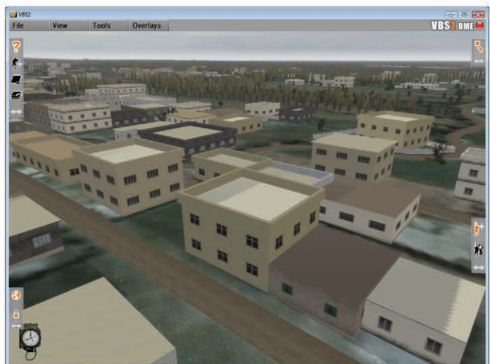
Buildings with parametric generation of roof structures
